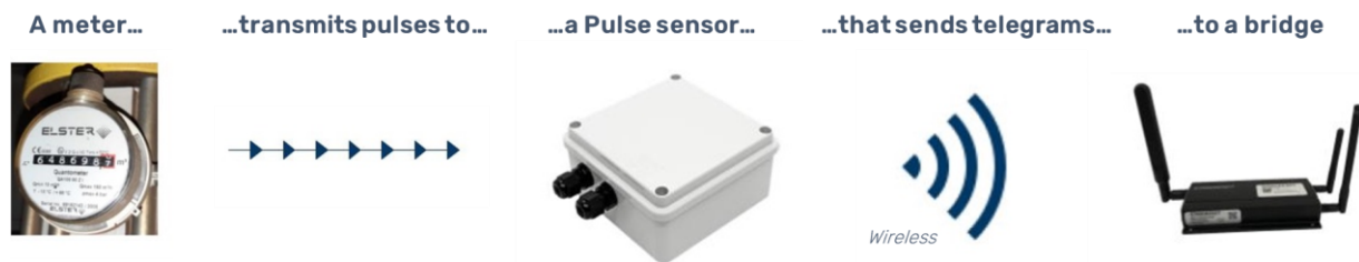
Basic functionality of the pulse sensor
