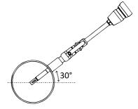
The VPSensorCartridge has a flow direction indicator, this also indicates the alignment of the instrument. A second indicator can be found on the safety system. Make sure it points in the right flow direction. Alignment "by the eye" is sufficient.
