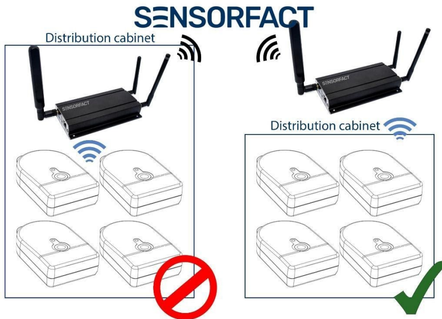
Figure 2.6 – Do not place the bridge in a distribution cabinet, this may disrupt the connection to the WiFi network or the mobile data network (4G).
